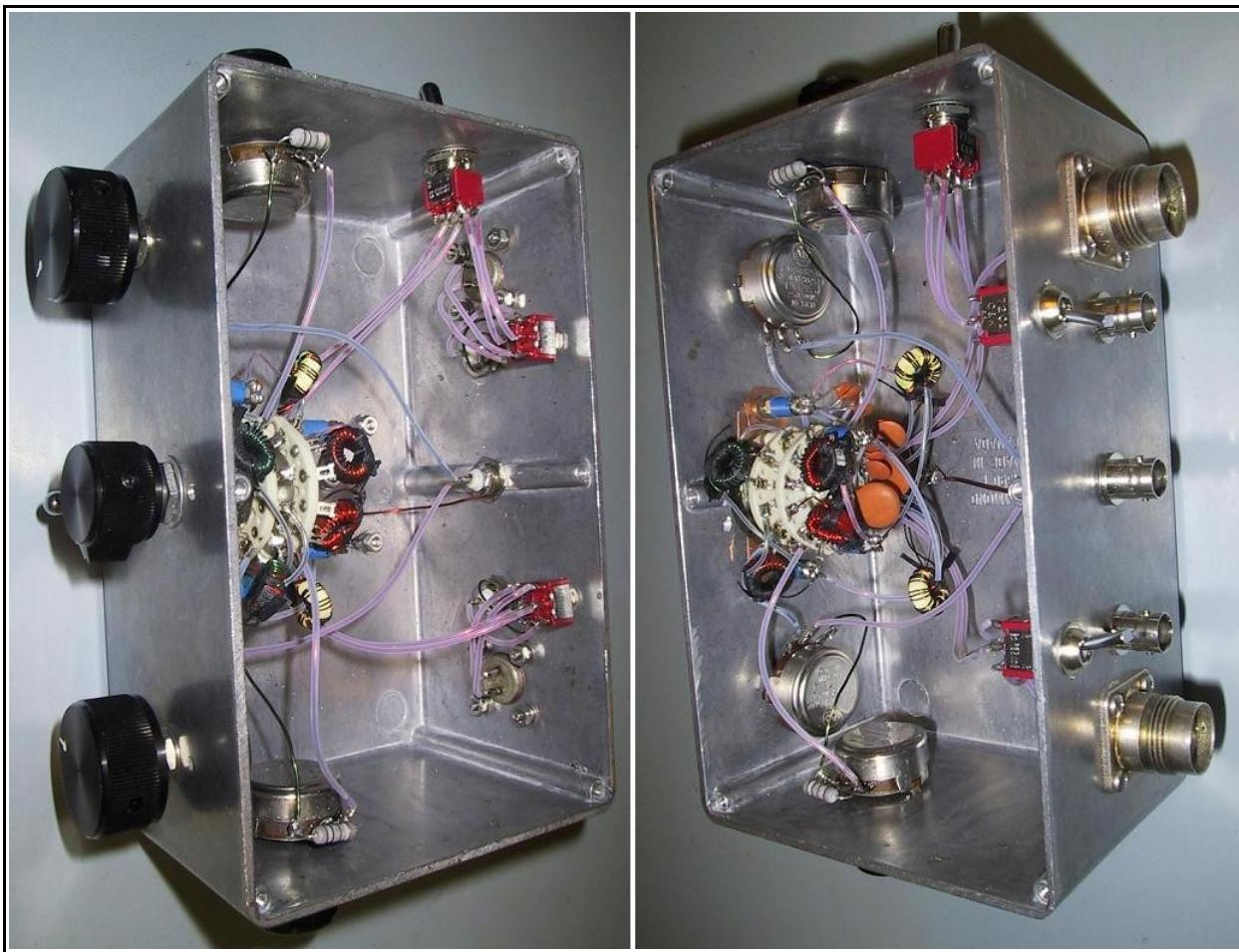
Above are interior photos of a previous version of the bandswitched 100 kHz – 30 MHz Passive Phaser. The switched inductive coupling enhancement (switch S5) was not implemented in this version. The vernier pots on
