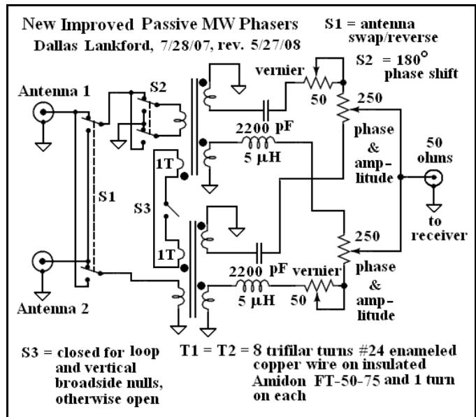
by Misek phasers. The new passive phasers described here are also not symmetric. But the asymmetry is different from the Misek asymmetry; not only is signal from an inductive phase shifted component routed to a capacitive phase shift component, but also signal from a capacitive phase shifted component routed to an inductive phase shifted component.
